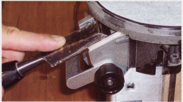
GETTING THE CORRECT ANGLE is foolproof: Set the guide to 20°, 25°, 30° or 35° and push the tool into the abrasive disk.
